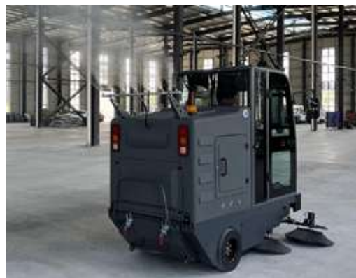
Dust Suppression with Water Spraying
