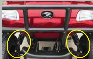
4 Tires with Shock Absorber System
